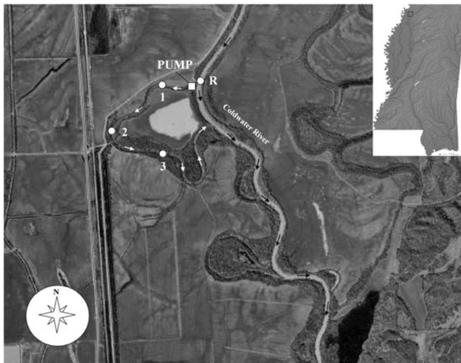
Figure 1. Aerial photograph of the backwater artificial flooding project along the lower Coldwater River, Mississippi. Arrows indicate water flow direction. Numbered symbols indicate water quality monitoring/sampling sites. Pumps were located at the white square.
